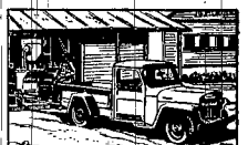
Belt power: With power take-off, it serves as a power unit for operating many types of belt-driven equipment.
